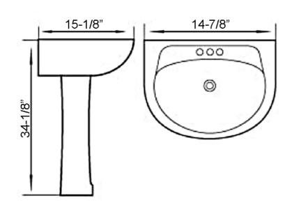
Dimensions of fixture are nominal and may vary within the range of tolerances established by ASME Standard A112.19.2.2018. Dimensions and specifications subject to change without notice.
